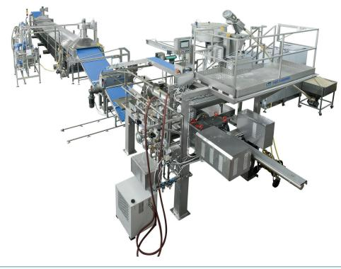
Another improvement is that one referring to the prevention of dough wrinkles or air bubbles; these are problems that can cause the dough to be sideslipped or sometimes torn. A belt with herring-bone rods has been designed to keep the dough just below the cooking water level. This solution prevents the dough to move sideways during the passage through the cooker whereas the air bubbles, pushed by the herring-bone rods, come out sideways.
